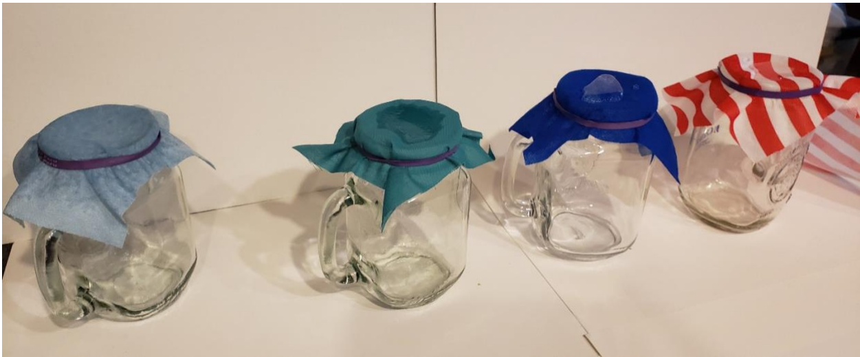
Figure 2. Home test of fluid penetrance, evaluating the amount of water transferred across each fabric over a 60 second time course with 5 ml water applied to each material. Left to Right: Blue Shop Towel (cellulose based; 1.75 ml collected inside jar), Cotton (3.75 ml collected), NWPP shipping bag (midweight; 0 ml collected), and NWPP shipping bag (heavier weight, 0 ml collected). Note the visually observable differences between water atop hydrophilic materials and hydrophobic materials.
