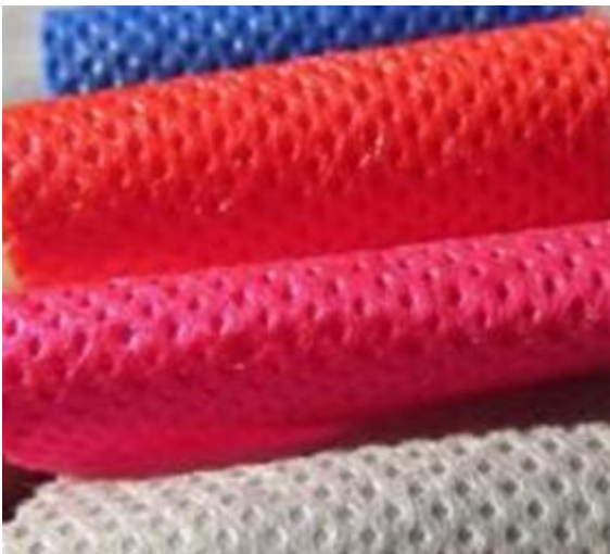
Figure 1. The characteristic diamond-shaped, dimpled pattern seen in spunbond NWPP
